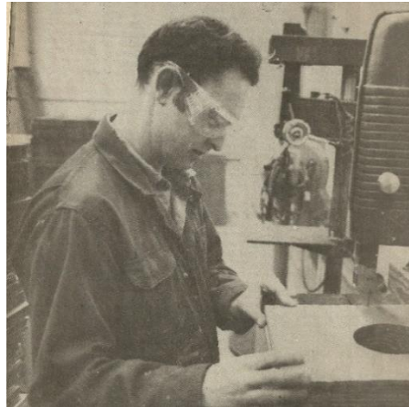
Jerry Manus custom cuts cardboard on the band saw and shapes it to fit customer specifications.
